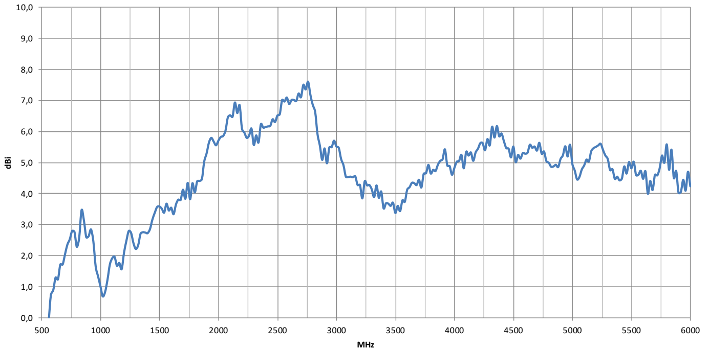
Antenna Peak Gain (dBi) by Frequency (Mhz)
